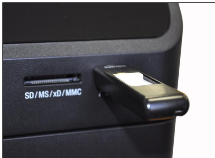
Above: The built-in memory interface located on the right side of the device lets users scan to a USB flash drive or memory card for instant portability
