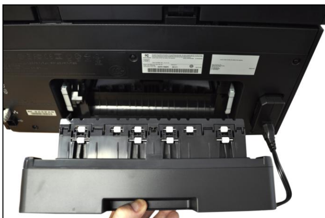
Above and below: Misfeeds can be cleared in the rear duplex area by removing the back cover and clearing any misfeeds.
