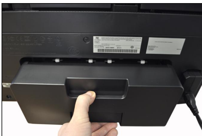
Above and below: Misfeeds can be cleared in the rear duplex area by removing the back cover and clearing any misfeeds.
