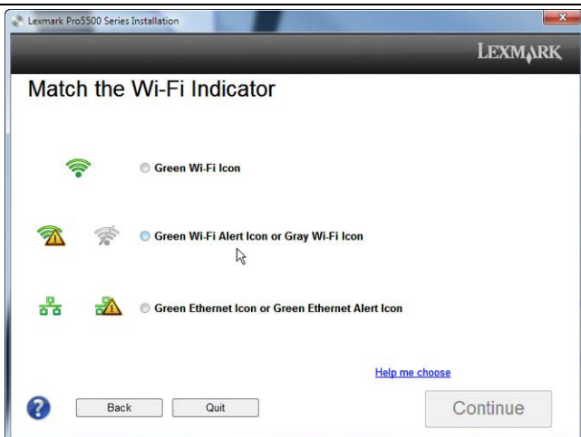
For wireless installation, match the icon on the control panel to the examples shown above.
